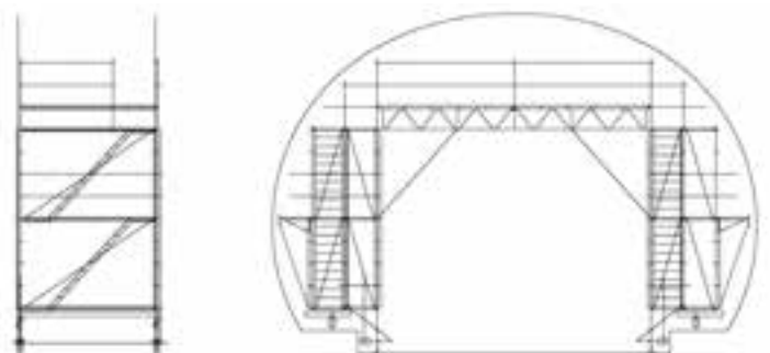
Mobile tunnel scaffolding
