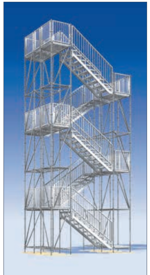
Stairway dimensions: riser s = 20.00 cm; tread a = 27.50 cm; undercut u = 4.50 cm
